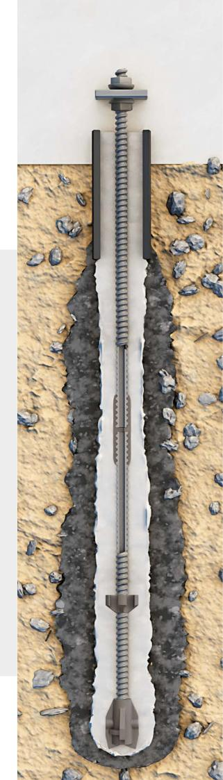
TITAN micropiles comply with EN 14199 "Execution of special geotechnical works – micropiles" and in Germany their use is regulated by National Technical Approval / Construction Technique Permit Z-34.14-209 issued by the German Institute of Building Technology (DIBt).
