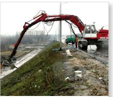
Excavator-mounted drilling equipment with hydraulic drive
